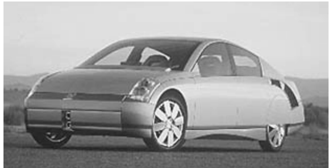
The GM Precept, a concept fuel cell vehicle, is projected to get over 100 mpg and carries hydrogen fuel onboard.
